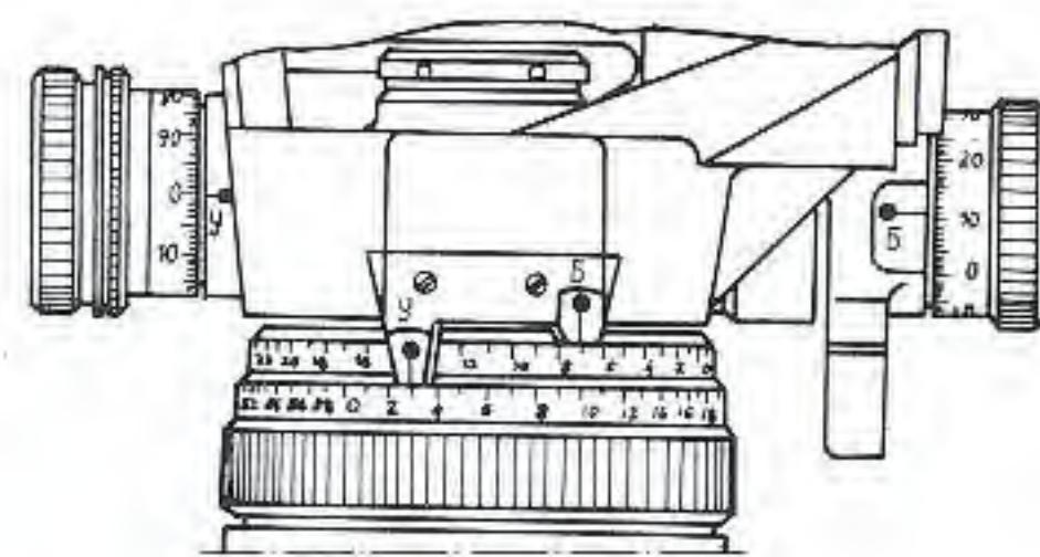
Sl. 16 – PRIMER OČITAVANJA MAGNETSKOG AZIMUTA  $Azm = 7-11.$
